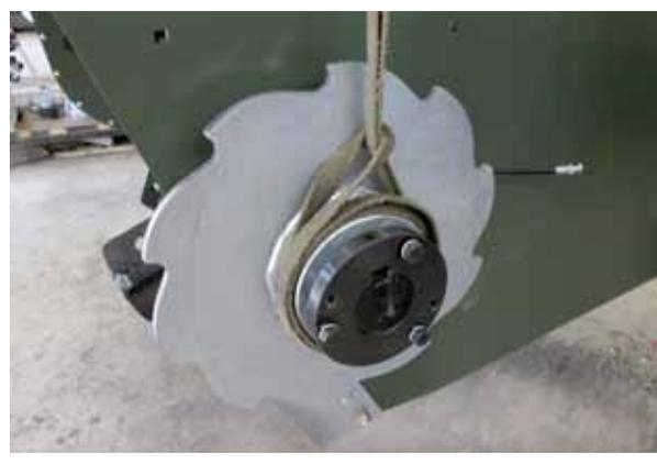
FIG 9-3 MOUNT SPROCKET
