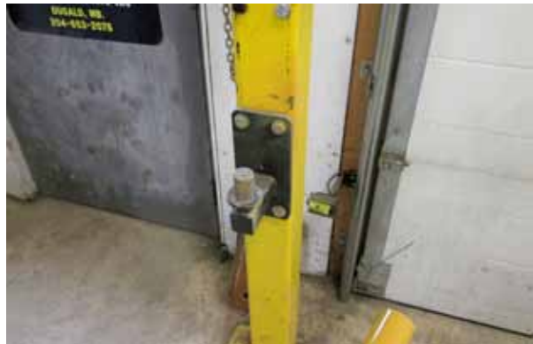
Stud Shaft (Typical)
